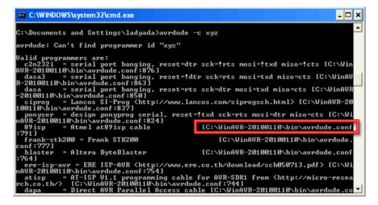
A common reason for wanting to program an AVR is to put the Arduino bootloader on there, in which case, you may not have WinAVR installed. Luckily, avrdude is there, its just 'hidden' in the IDE package (for Mac users, you need to actually "explore" the App) if you're running windows, go to the folder where you have the IDE installed and go into the hardware\tools\avr\etc folder to open up avrdude.conf
